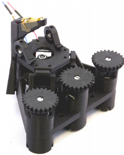
FIG. 1. Photograph of the microscope. The three gears at the front control lateral motion (outer gears) and focus (centre), while the sample is held on the translating stage by two printed clips. A white LED is mounted on a printed arm at the top, and the lens (from the Raspberry Pi camera module) is visible through the hole in the sample stage. The camera sensor mounts underneath the microscope.
